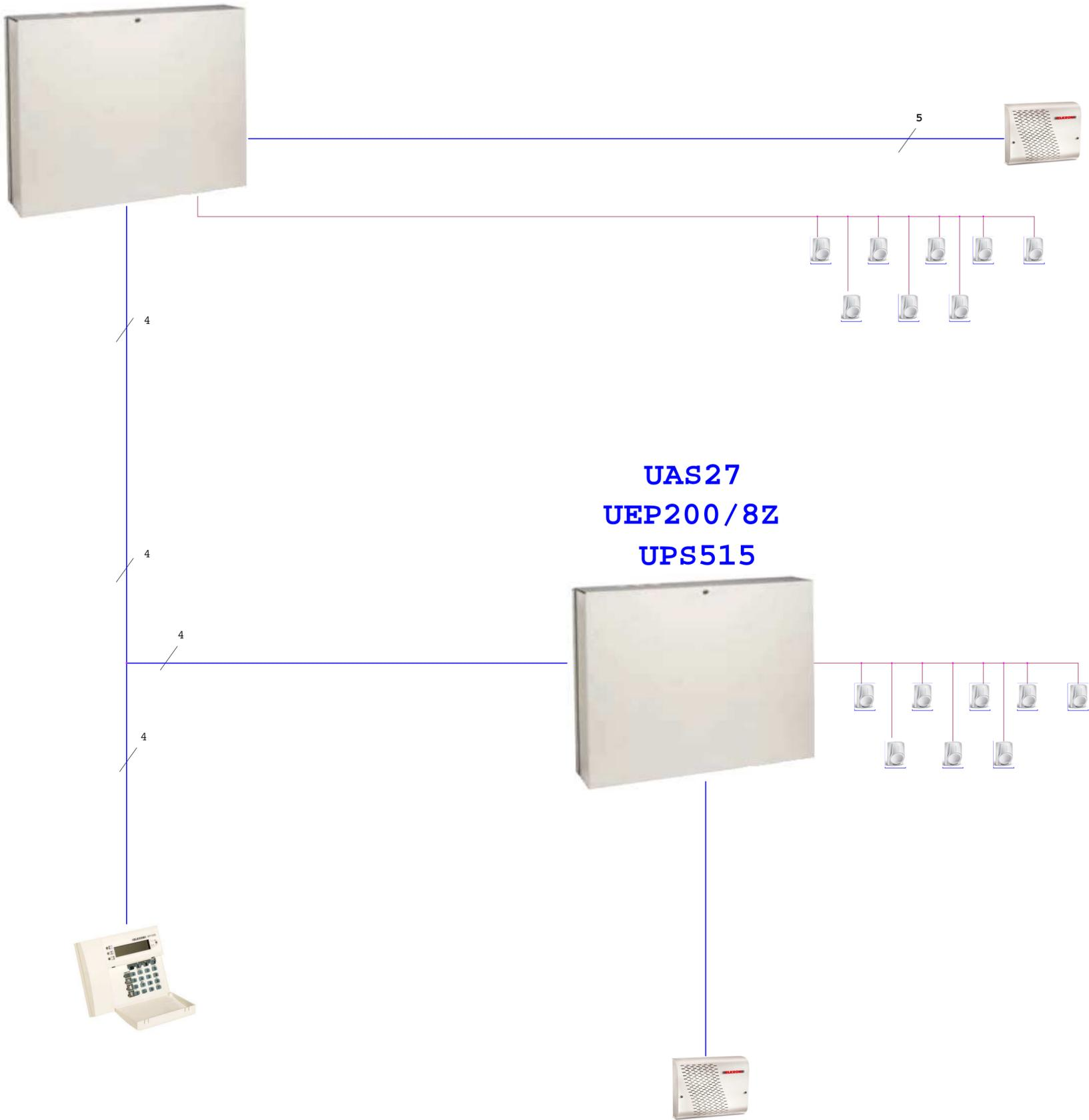
UMP508 EXEMPLE DE CABLAGE AVEC 3 BUS
