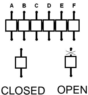
Cutting of the jumpers marked by an asterisk (\*), will imply the loss of conformity with EN50131 standards.
