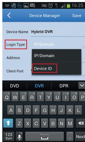
2. Fill in the field “Device name” and then select “Type” → “Device ID”.
