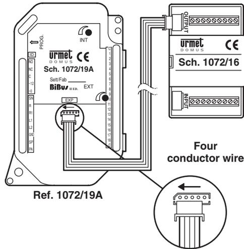
**N.B.:** *The buttons associated to the expansion modules will not send the call if the wire is not inserted correctly.*
